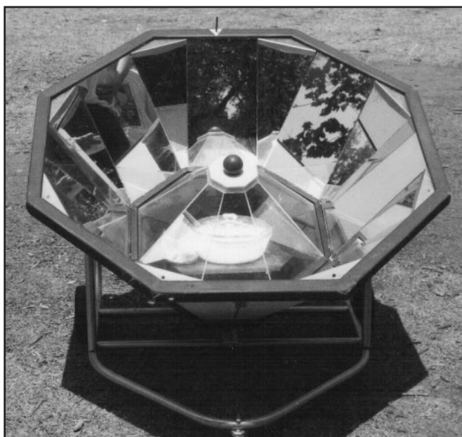
Figure 4 Concentrator Oven Combining high concentration with an insulated cooking compartment can deliver excellent performance
