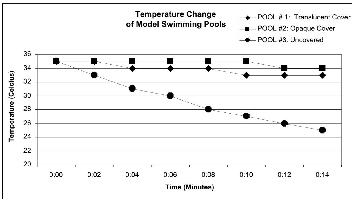
Figure 1. Sample graph: Time vs. Temperature Measurement of Each Pool
