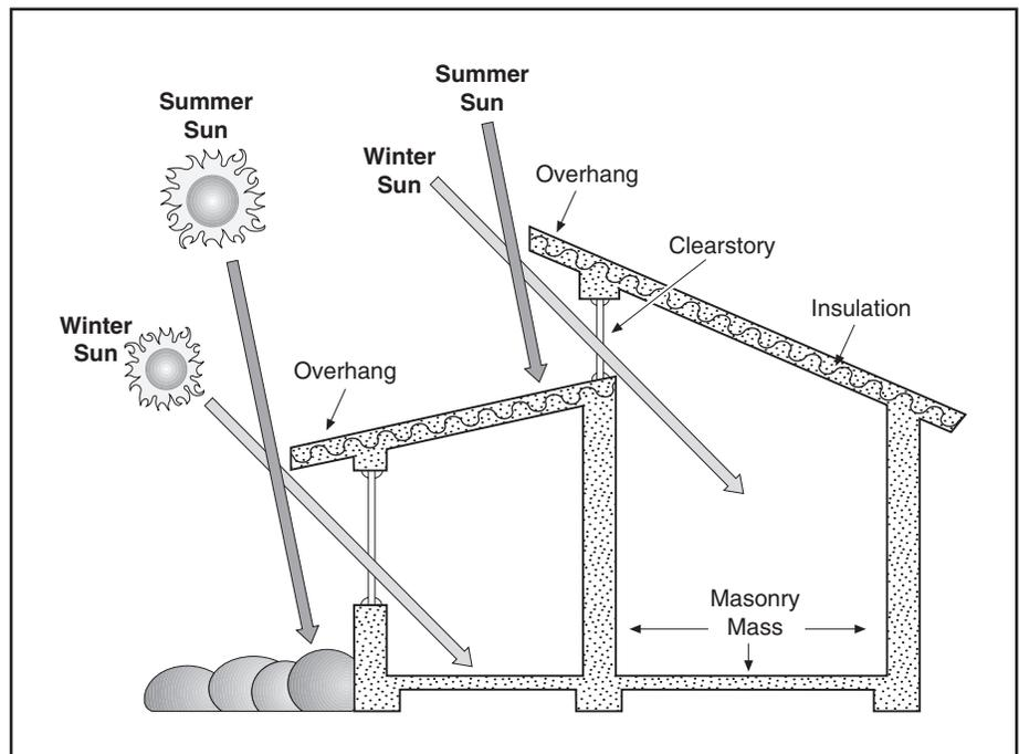
**Fig. 1. Sun angles** This cross-section illustrates the direct gain concept.
